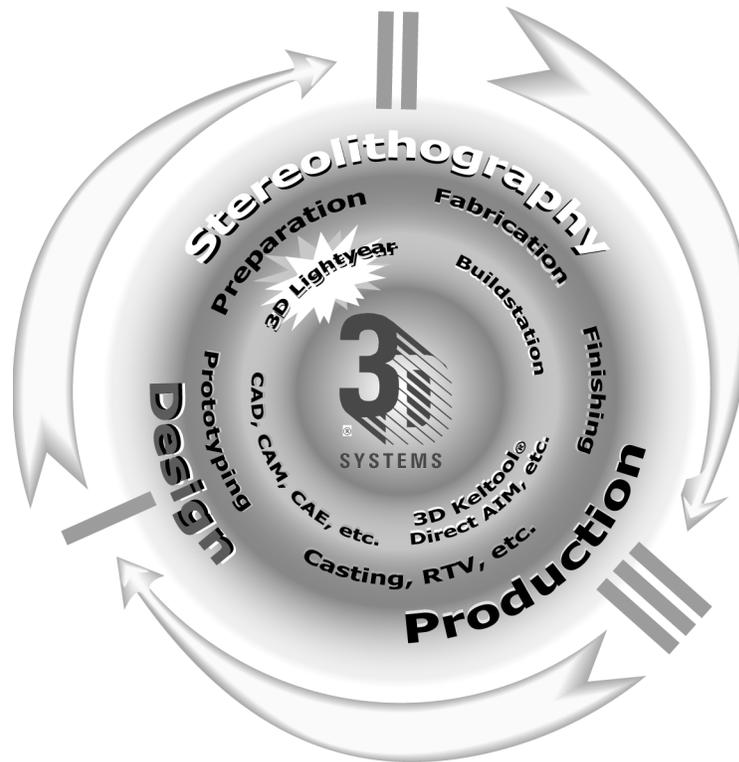
Figure 1. Stereolithography in the Product Development Process
