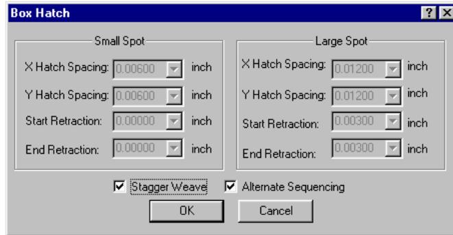
Figure 78. *Hatch Parameters, Standard SLA 7000 users*
