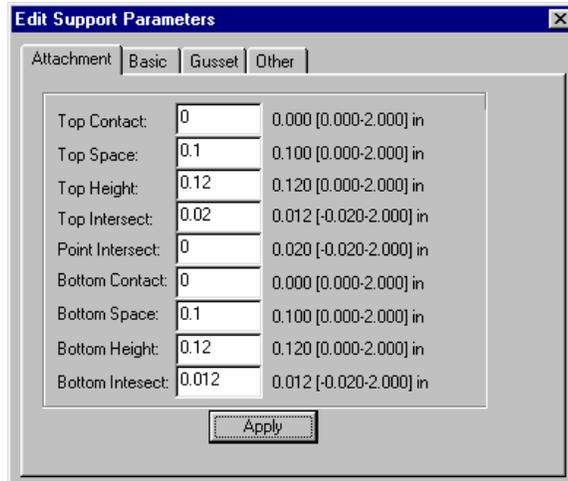
Figure 104. Edit Support Parameters Dialog Box (Attachment Tab)
