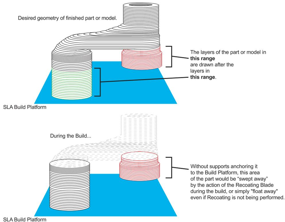
Figure 57. Supports and Anchoring
