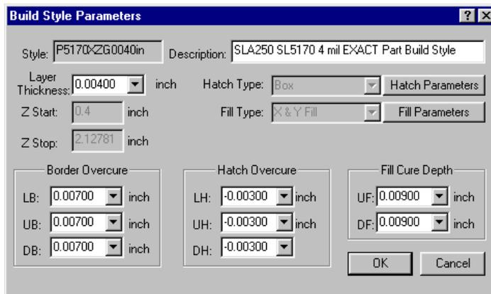
Figure 75. *Build Style Parameters Dialog, Standard SLA 190 and 250 users*
