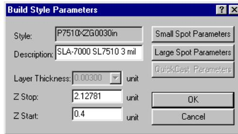
Figure 76. Build Style Parameters Dialog, Advanced SLA 7000 users
