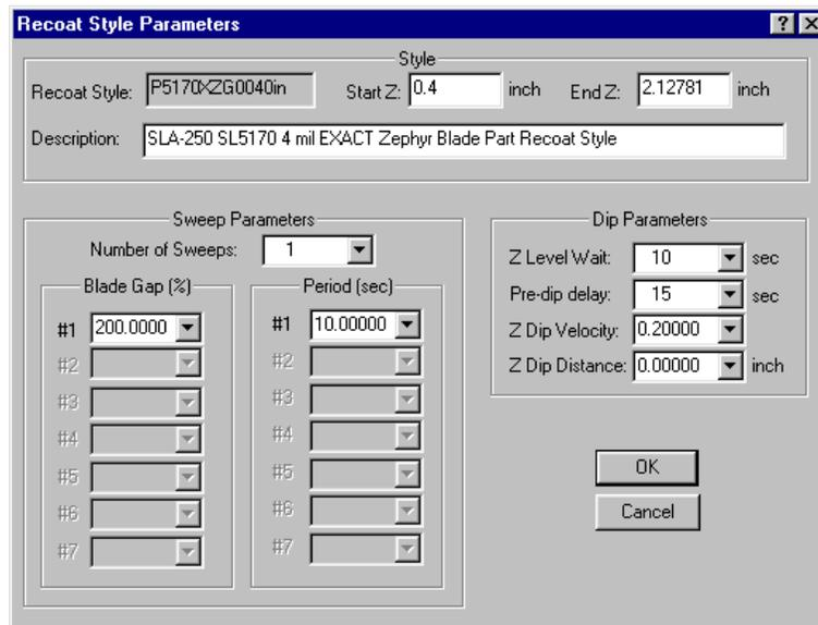
Figure 92. *Recoat Style Parameters Dialog, SLA 250 users*
