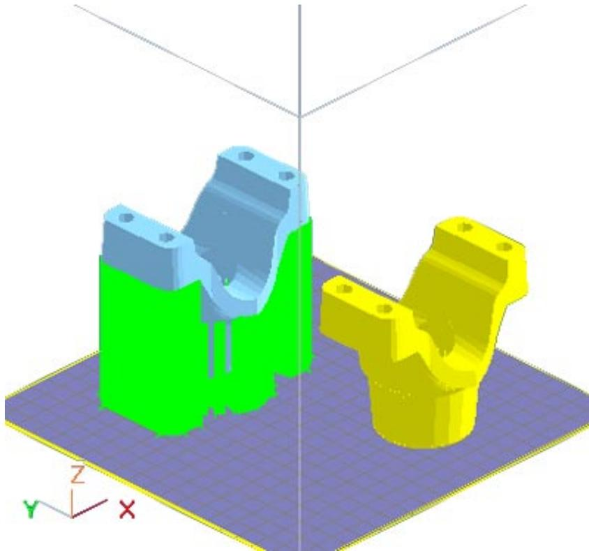
Figure 60. Build Platform (one part with Supports, and one without)
