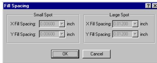
Figure 79. *Fill Spacing Parameters, Standard SLA 7000 users*
