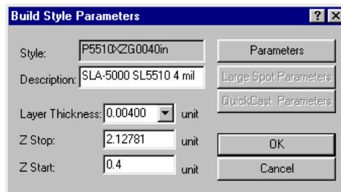
Figure 77. Build Style Parameters Dialog, Advanced SLA 190, 250, 350, 500, 3500, and 5000 users
