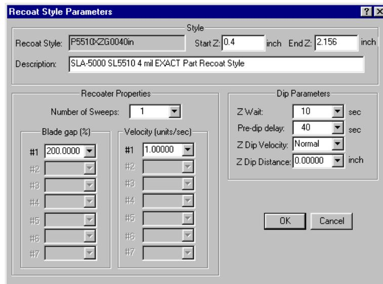
Figure 91. *Recoat Style Parameters Dialog, SLA 350, 500, 3500, 5000, and 7000 users*
