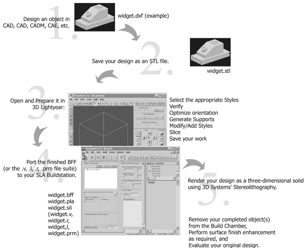
Figure 2. Stereolithography Process Flow
