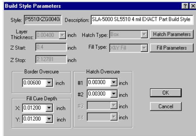
Figure 74. *Build Style Parameters Dialog, Standard SLA 350, 500, 3500, and 5000 users*
