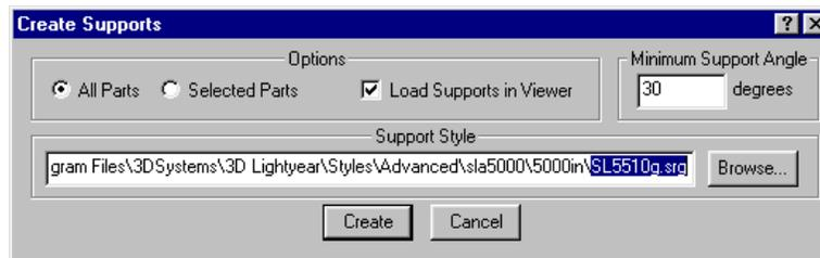
Figure 116. Create Supports Dialog with Minimum Support Angle
